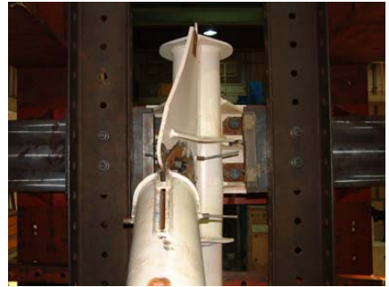
Figure 5(c). Gusset Pl. Buckling in TC-1
